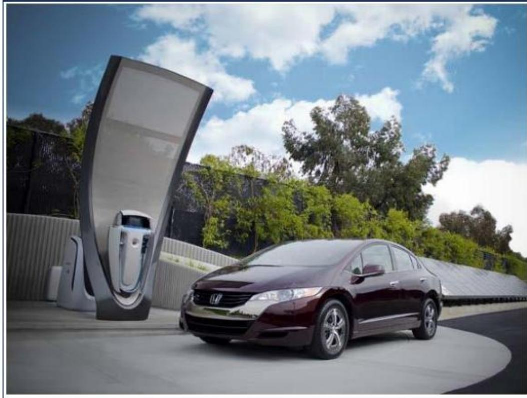
Honda's New Solar Hydrogen Fueling System (Source: Honda Motor Company, 2010)
